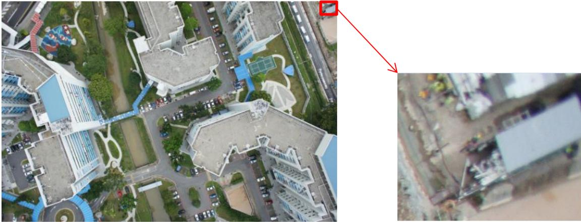
**Figure 3:** Blur in image corners of Sony Nex-5
